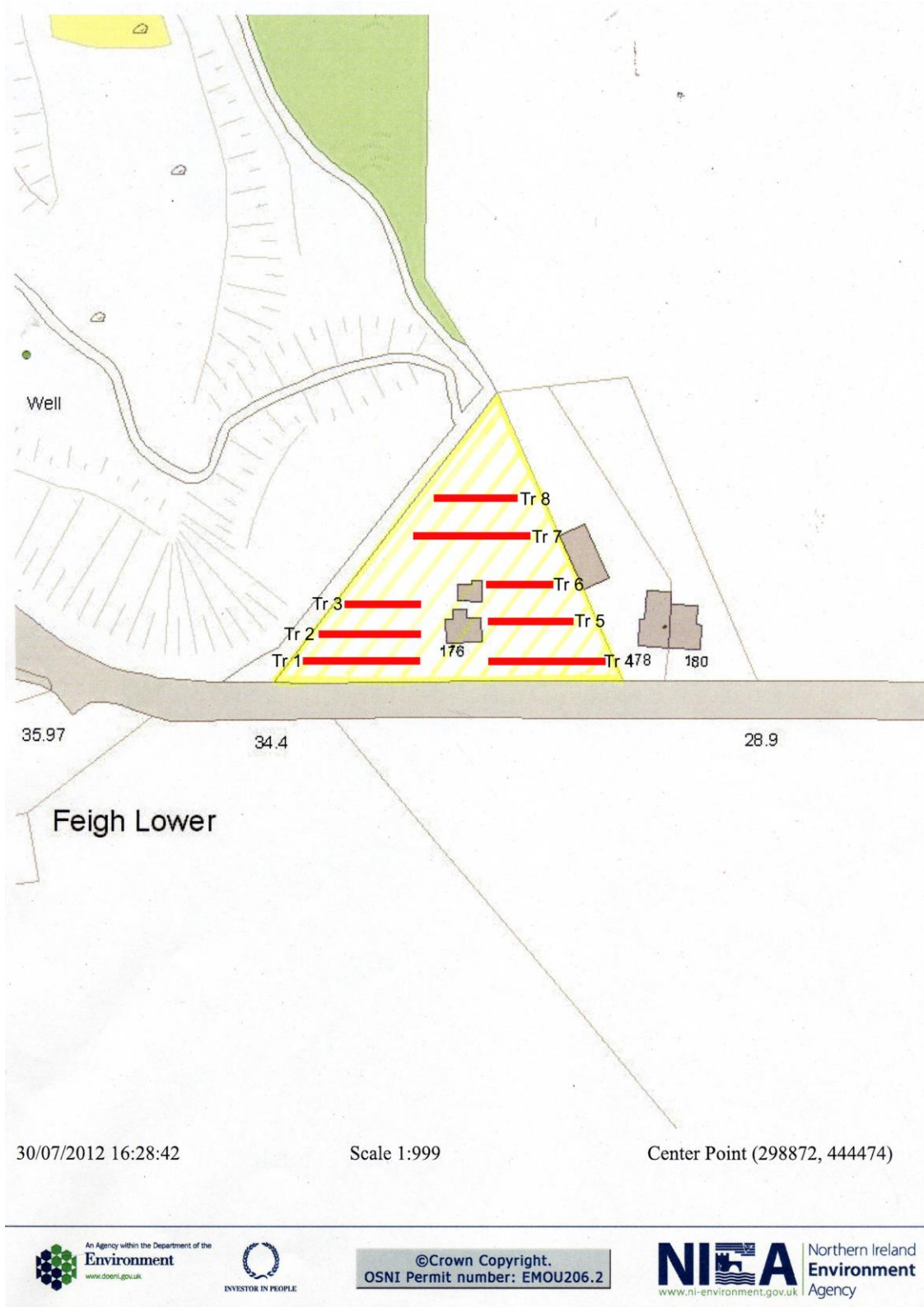
Figure 3: Site plan showing location of test trenches
