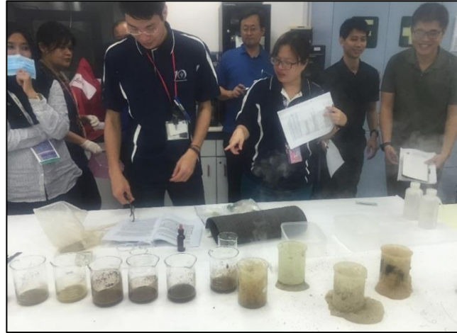
Fig. 6. (Left) Participants assisting Rob Fitzpatrick to sample Acid Sulfate Soils in Acid Sulfate Soils in the SungeiBuloh Mangrove Wetland Reserve on Friday 9th September. (Right) Participants conducting pH measurements in water and after peroxide treatment on a range of acid sulfate soils sampled in the SungeiBuloh Mangrove Wetland Reserve.
